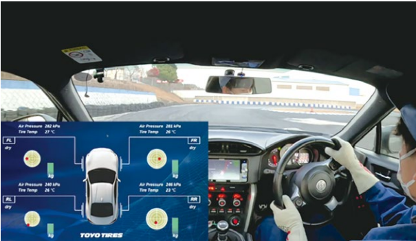
The app screen visualizes tire force during driving
