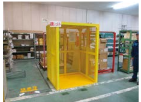
Temporary shelter for use in the event of an earthquake (Kuwana Distribution Warehouse)
