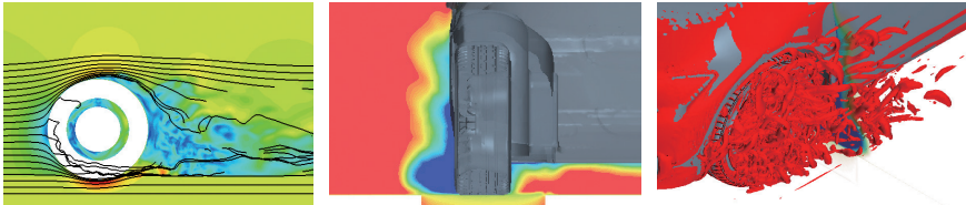
Visualization of air resistance using “Mobility Aerodynamics” (aerodynamic simulation) technology
