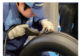
A demonstration on hand-carving a tire (Showa Estate Co., Ltd.)
