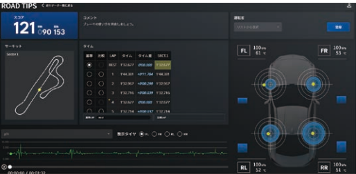
Application displaying visualization of tire force in a run
